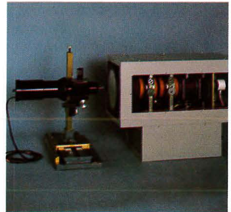
CELCO CRT Spot Analyzer, CRT Display, w/Deflection Yoke, Focus Coil, Lens Assemblies, Correction Circuits, Micro-positioners and Magnetic Shielding.
